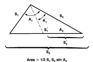
\* Note that two possible solutions exist if  $S_2$  is greater than  $S_1$  and  $A_3$  does not equal 90°. Both possible answer sets are calculated.
