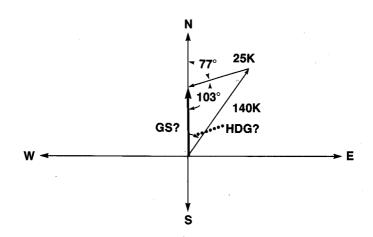
By subtracting the wind direction from 180 (yielding an angle of  $103^{\circ}$ ), the problem reduces to a  $S_1$ ,  $S_2$ ,  $A_2$  triangle.
